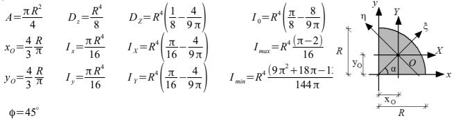
NOTE:  $D_z$  and  $D_z$  are calculated for an orientation of the quarter as in the figure.
