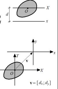
**NOTE**:  $d_x, d_y$  may be negative! While in case of moments of inertia it is not important as we square d anyway, in case of deviation moment of inertia accounting for a sign of  $d_x, d_y$  is necessary.  $d_x, d_y$  Are components of vector of translation of coordinate system – however it may be chosen arbitrary if this is a vector from the old coordinate system to the new one or in the opposite way.
