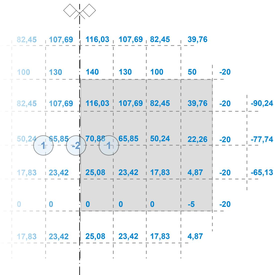
$$\begin{aligned}\sigma_{xx} &= \frac{\partial^2 F}{\partial y^2} \approx \frac{1}{s^2} (F_{21} - 2F_{31} + F_{41}) = \\ &= \frac{1}{1^2} (25,08 - 2 \cdot 70,88 + 116,03) = -0,65 \text{ kPa}\end{aligned}$$
