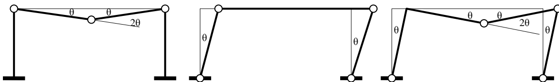
Fig. 15.10 Kinematical schemes of collapse
