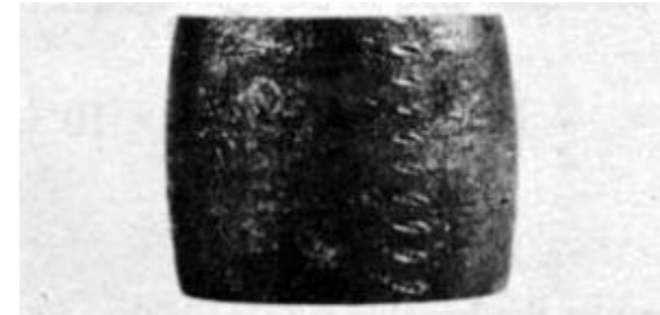
Barrel-like failure of compressed mild-steel specimen
