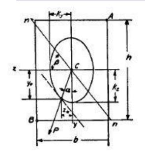
the neutral axis:  $z = \tan \alpha \cdot \frac{l_y}{l_z} y$ , the inertia ellipse equation:  $\frac{y^2}{i_z^2} + \frac{z^2}{i_y^2} = 1$ the equation of the tangent at the point  $(y_0, z_0)$ :  $\frac{yy_0}{i_z^2} + \frac{zz_0}{i_y^2} = 1$ the tangent of the angle between the *z* axis and this tangent will be:  $\frac{z_0}{y_0} \cdot \frac{i_z^2}{i_y^2} = \tan \alpha \frac{I_z}{I_y} = \tan \beta$
