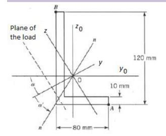
Plates are welded together to form the 120 mm by 80 mm by 10 mm anglesection beam shown in the Figure. The section is subjected to a bending moment 4.8 kNm, that lies in the plane making an angle  $\varphi = \frac{2}{3}\pi$  with the x-z plane. Determine the maximum tensile and compressive bending stresses. Solution
