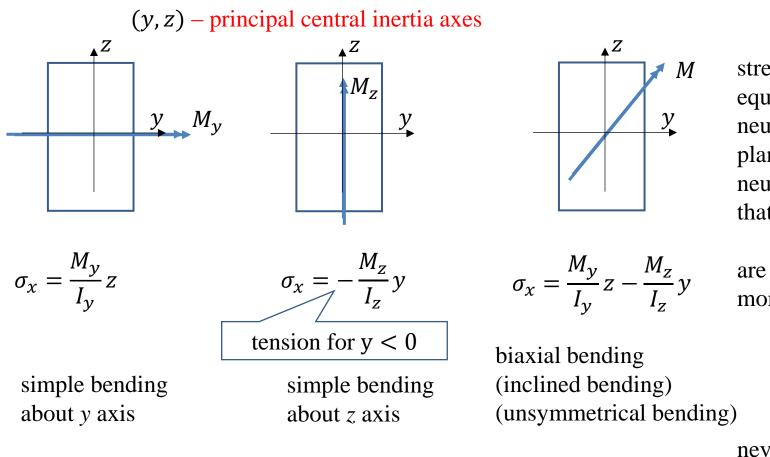
stress distribution is given by the equation of plane neutral axis: intersection of the c-s plane and the stress plane neutral axis is a straight line that passes by the c-s centroid
