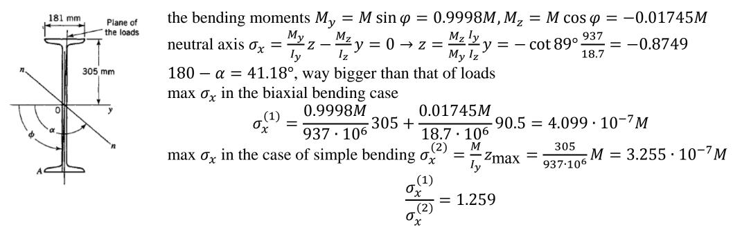
The maximum stress in the I-beam is increased 25.9% when the plane of the loads is merely 1° from the symmetrical vertical plane. This section should not be used as beam unless the lateral deflection is prevented.
