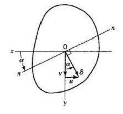
The total deflection  $\delta$  of the centroid at any section of the beam is perpendicular to the neutral axis.
