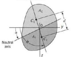
Prandtl's schematization with the yield point  $\sigma_0$  in both tension and compression because N = 0, the neutral axis divides the cross-section in half,  $A_t = A_c$ resultant of tension stresses of  $A_t$  is applied at the centroid  $C_t$ resultant of compression stresses of  $A_c$  is applied at the centroid  $C_c$ these resultants form a couple of forces:  $M = \sigma_0 A_t d = \frac{\sigma_0 A d}{2}$ the centroids of the cross-section halves lie on the action axis
