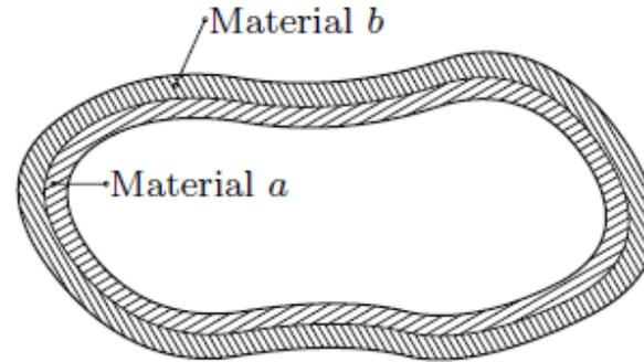
The Bredt's formula is valid only in terms of stress flow:  $f = \tau_a \delta_a + \tau_b \delta_b = \frac{M_x}{2A}$ ,  $A$  – area limited by the center line of the composite section. As the distortion must be the same in the two materials, we have:
