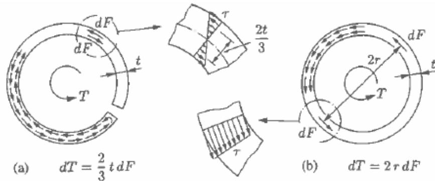
correction of the Bredt's formulas by breaking cross-section into closed and open parts
