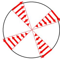
the stress vector is perpendicular to the radius and its length is
