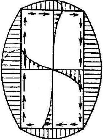
trigonometric series expansion for the distortion function  $\varphi = \sum_k^{1,3,5,\dots} f_k(y) \cos \frac{k\pi y}{a}$
