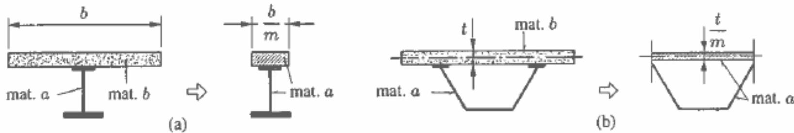
Equivalent cross-sections for the composite beams made from materials  $a$  and  $b$
