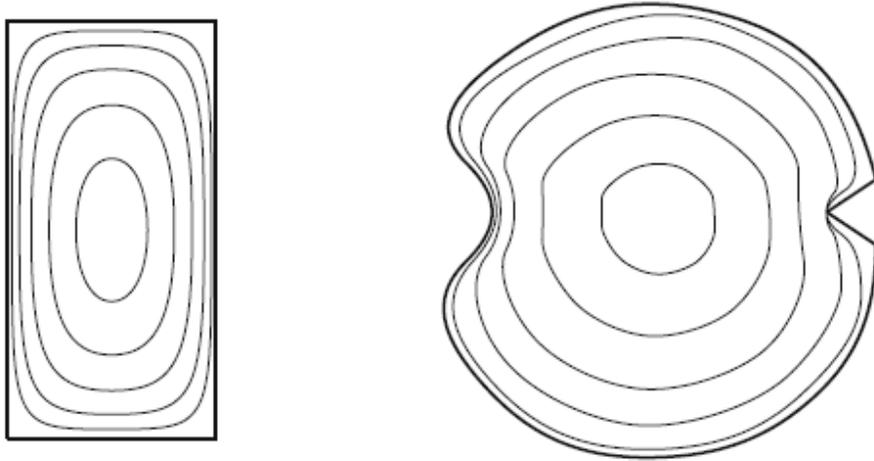
the volume of the solid between the Prandtl's function and the cross-section plane is proportional to the torque
