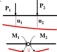
Corresponding generalized displacement is the sum of displacements  $u_1+u_2$
