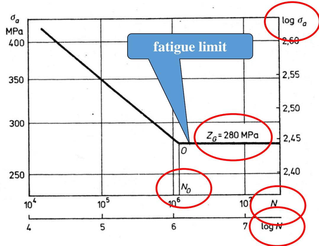
Wöhler's diagram for high-cycle fatigue
