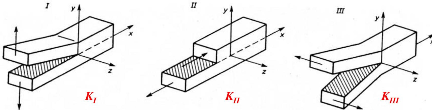
Mode I – opening; the crack surfaces move directly apart (a tensile stress normal to the plane of the crack).
