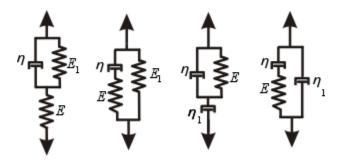
Answ.: for model VK-H  $(E_2, \eta - E_1)$ :  $\eta \dot{\sigma} + (E_1 + E_2)\sigma = E_1\eta \dot{\varepsilon} + E_1E_2\varepsilon$ (instantaneous elasticity, limited creep, elastic return, full recovery)  $\sigma_{\uparrow}$
