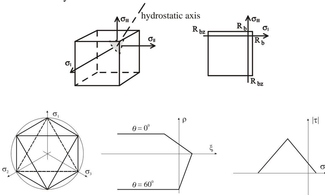
Fig. 2.7 Different views of Rankine's criterion
