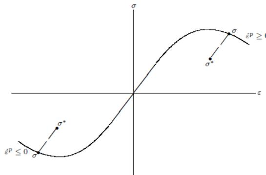
Fig. 2.4 Maximum-plastic-dissipation postulate (in uniaxial stress-strain plane)
