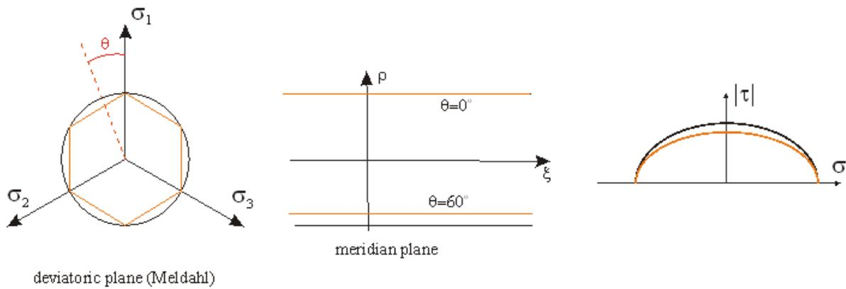
Fig. 2.10 Comparison of Tresca and Huber-Mises criteria
