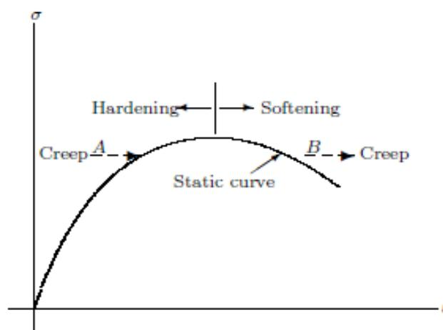
Fig. 2.1 Static curve<sup>1</sup>
