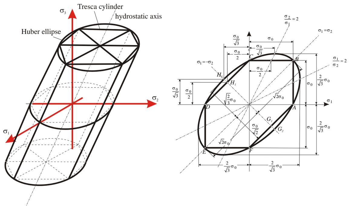
Fig. 2.9 Comparison of Tresca and Huber-Mises criteria
