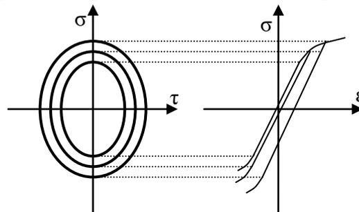
Fig. 2.16 Plastic isotropic hardening
