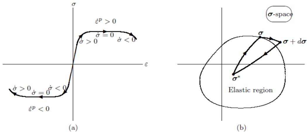
Fig. 2.3 Drucker's postulate: (a) in uniaxial stress-strain plane;(b) in stress space<sup>3</sup>
