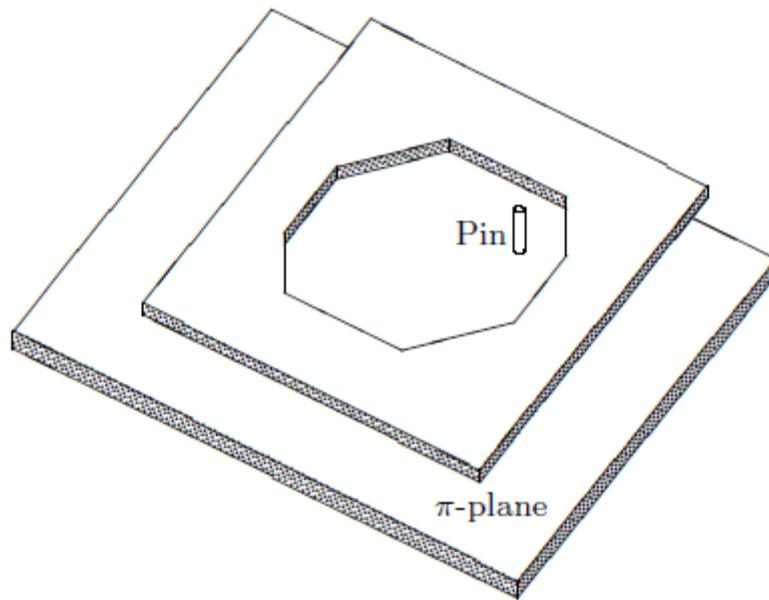
Fig. 2.17 Prager’s mechanical model of kinematic hardening
