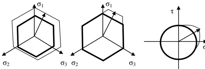
Fig. 2.19 Different mechanisms of anisotropic hardening
