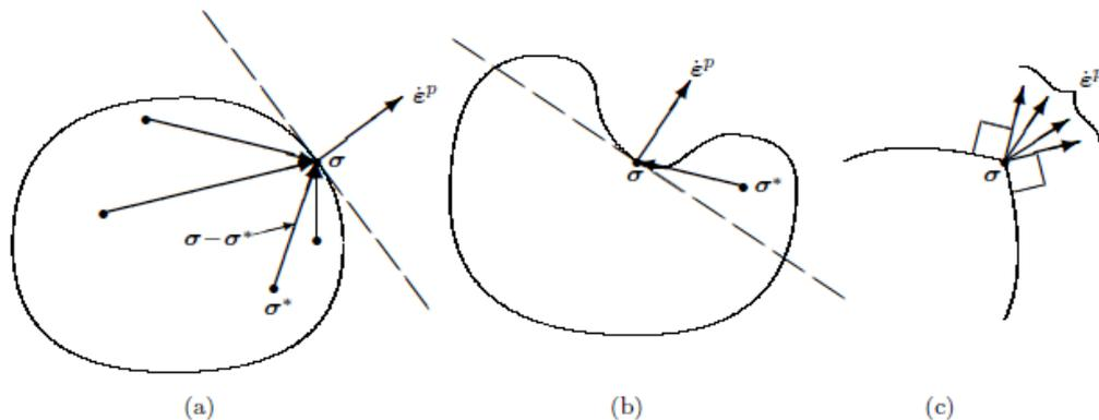
Fig. 2.5 Yield surface with associated flow rule: (a) normality; (b) convexity; (c) corner
