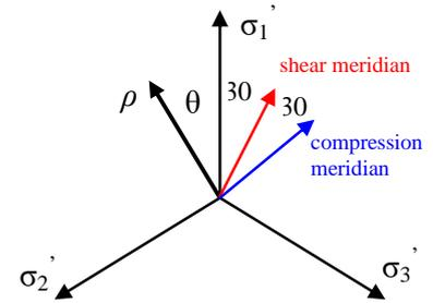
Fig. 2.8 Shear and compression meridians
