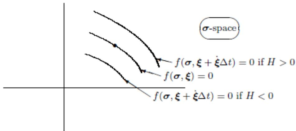
Fig. 2.2 Hardening and softening in rate-independent plasticity<sup>2</sup>
