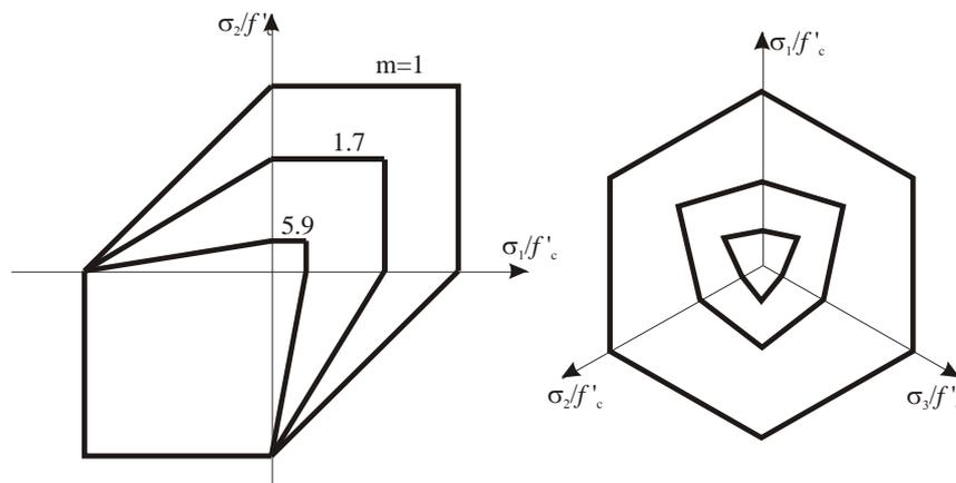
Fig. 2.14 Mohr-Coulomb criterion for different tensile/compressive yielding ratio
