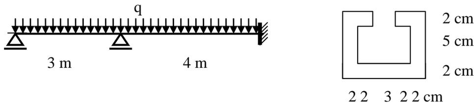
Fig. 3.20 Beam and the cross-section
