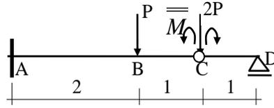
Fig. 3.11 Scheme with the hinge at C
