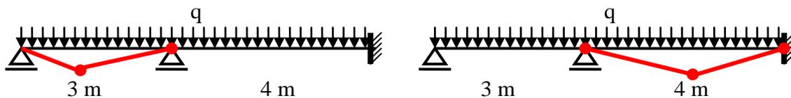
Fig. 3.23 Kinematic scheme
