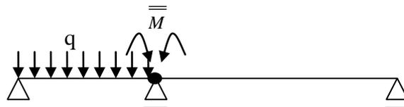
Fig. 3.17 Beam with the hinge
