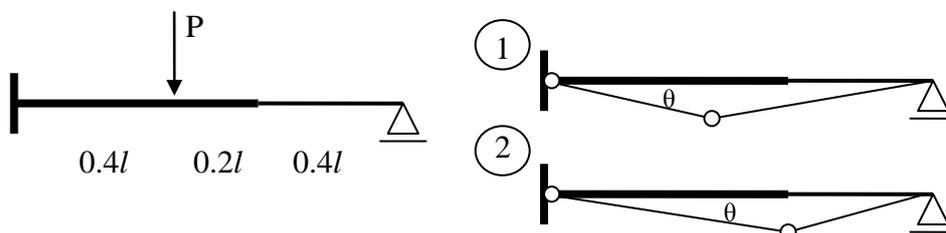
Fig. 3.15 Beam with variable stiffness and collapse schemes
