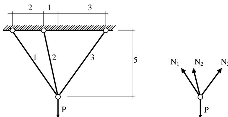
Fig. 3.6 Statically indeterminate truss and the node equilibrium
