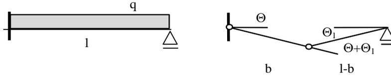
Fig. 3.13 Beam and the kinematic scheme of collapse
