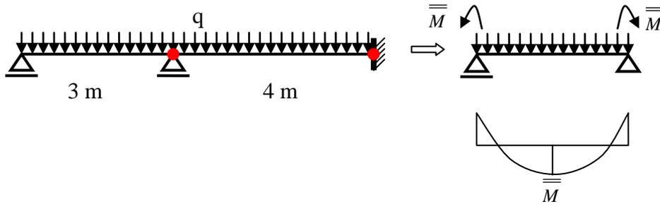
Fig. 3.22 Beam with two plastic hinges
