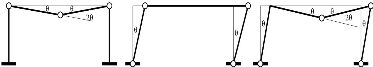
Fig. 3.38 Mechanisms of collapse
