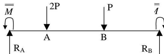
Fig. 3.32 Beam with two hinges
