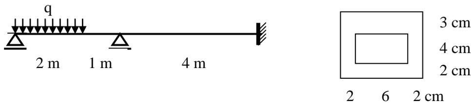
Fig.3.24 Beam with the cross-section
