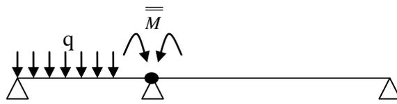
Fig. 3.25 Beam with the hinge
