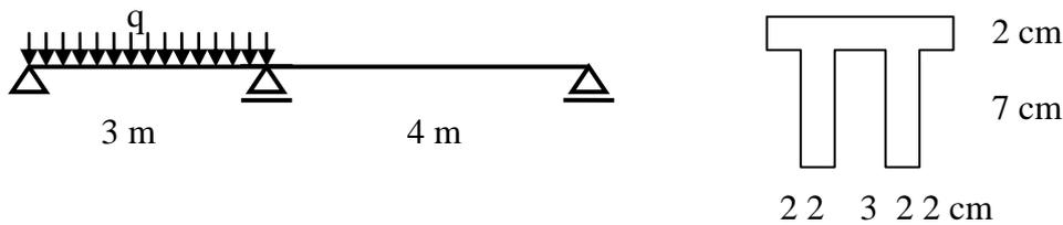
Fig. 3.16 Beam and the cross-section
