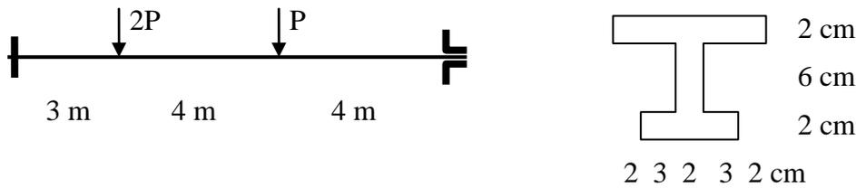
Fig. 3.31 Beam and the cross-section
