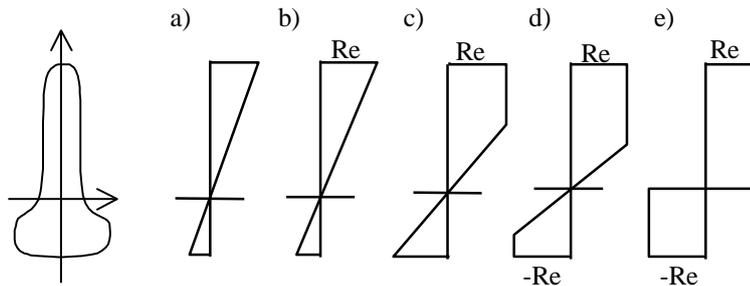
Fig. 3.1 Stages of the cross-section work
