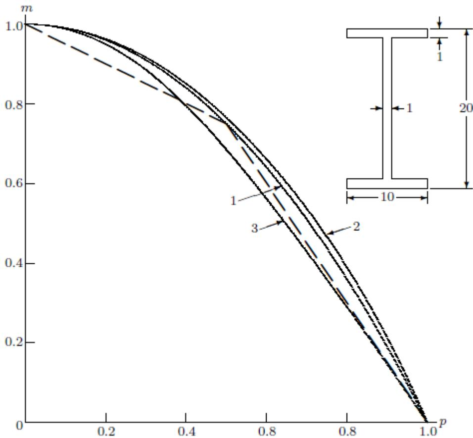
Fig. 3.4  $n$ - $m$  curves for rectangle (1), circle (2) and I-beam (3)
