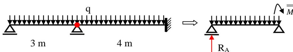
Fig. 3.21 Beam with the plastic hinge
