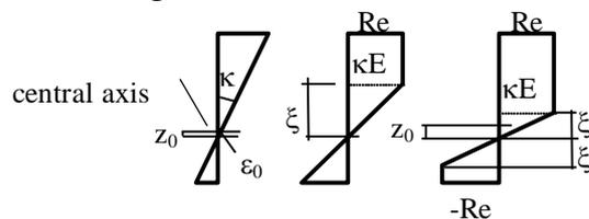
Fig. 3.2 Parameters of the stress distribution
