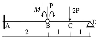
Fig. 3.10 Scheme with the hinge at B
