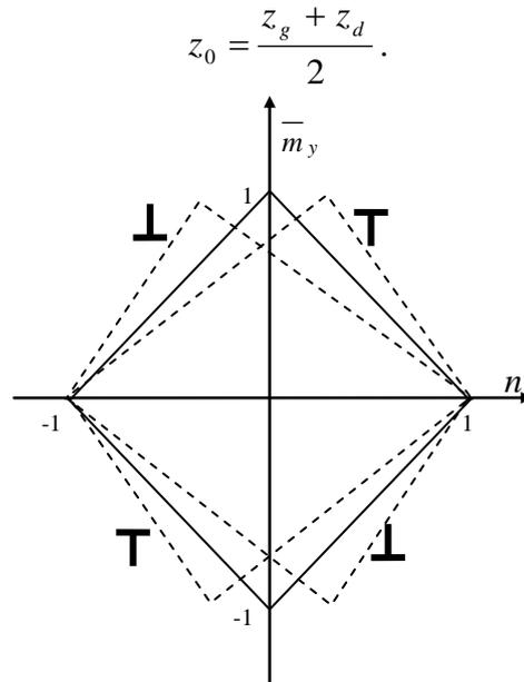
Fig. 3.3 Interaction curves of  $n - \bar{m}$
