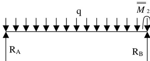
Fig. 3.29 Beam with the hinge
