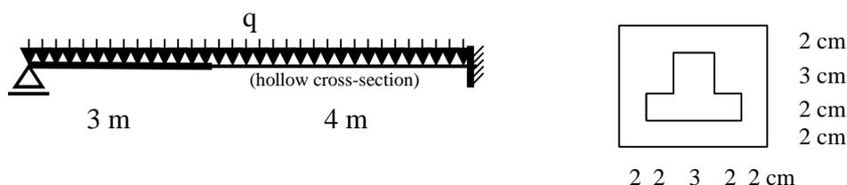
Fig. 3.28 Beam and the cross-section
