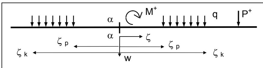
$$w_{\alpha-\alpha} = \frac{\alpha}{2k} \sum_{i=1}^n P_i \eta(\zeta_i) + \left[ -\frac{\alpha^2}{k} \sum_{i=1}^m M_i \eta_3(\zeta_i) \right]^* + \frac{1}{2k} \sum_{i=1}^r q_i [\eta_2]_{\zeta_p}^{\zeta_k}$$
