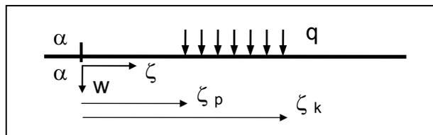
$$w_{\alpha-\alpha} = \frac{\alpha}{2bc} \int_{\zeta_p}^{\zeta_k} q_0 \frac{d\zeta}{\alpha} \eta(\zeta) = \frac{q_0}{2bc} \int_{\zeta_p}^{\zeta_k} e^{-\zeta} (\cos \zeta + \sin \zeta) d\zeta = \frac{q_0}{2bc} [\eta_2]_{\zeta_p}^{\zeta_k}$$
